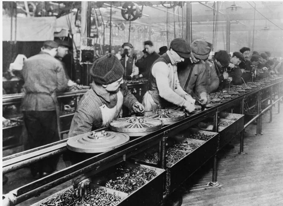
Henry Ford introduced the assembly line in 1913 to make the car assembly process more efficient.
