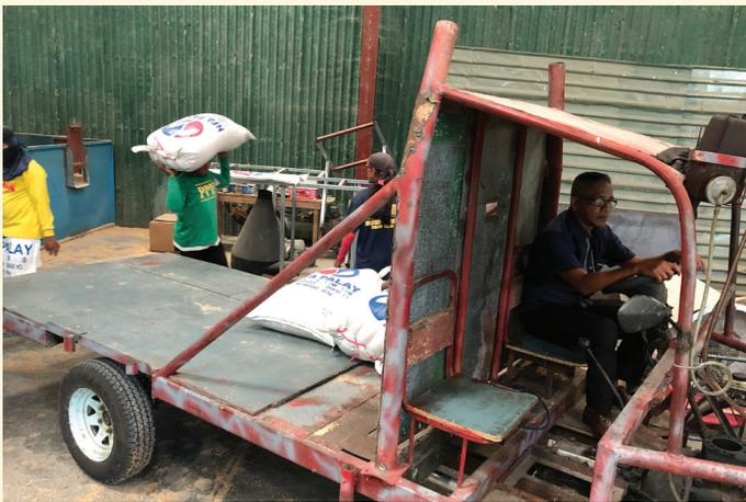
**S**crap materials and junk transmission engine declared for disposal lay idly around the compound of the National Food Authority (NFA) in Dumangas, Iloilo. One employee saw the value of these materials, tinkered with them, and was able to assemble a utility vehicle which saved for the agency millions of pesos in handling expenses. This is the story of Pepito P. Pauchano, a mechanical plant operator in NFA.
